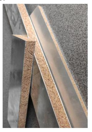
Cork products are suggested for interior design of aircraft. Moreover, some applications are about replacing metallic parts in wings such as spars or ribs with cork based sandwiches.
